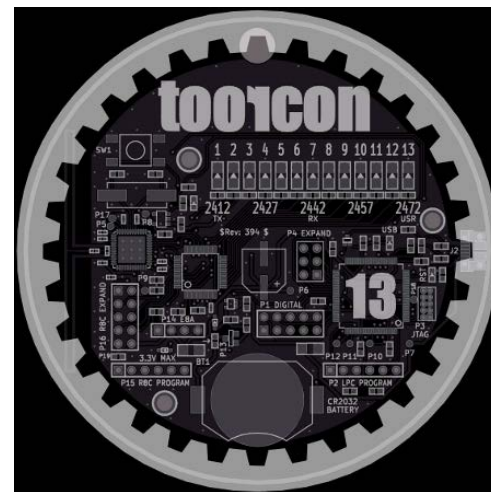
RF spectrum analyzer with LEDs representing 13 evenly spaced Wi-Fi channels in the 2.4 GHz band
